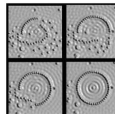
Quantum corral of 48 iron atoms on copper surface
